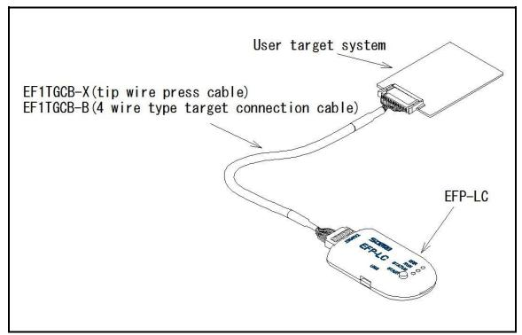
Fig3.1 Connection with target system
