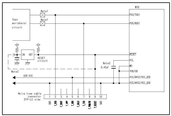
Fig5.1 User Target Peripheral Circuit Example (For RX66T)
