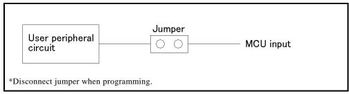
Fig5.2 Collision Prevention Circuit Using Jumper
