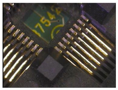
Fig 10 State where contact failure has occurred
