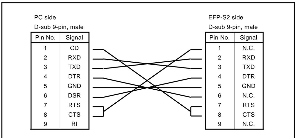
Fig. 4.1: RS-232C Cable Connection Diagram
