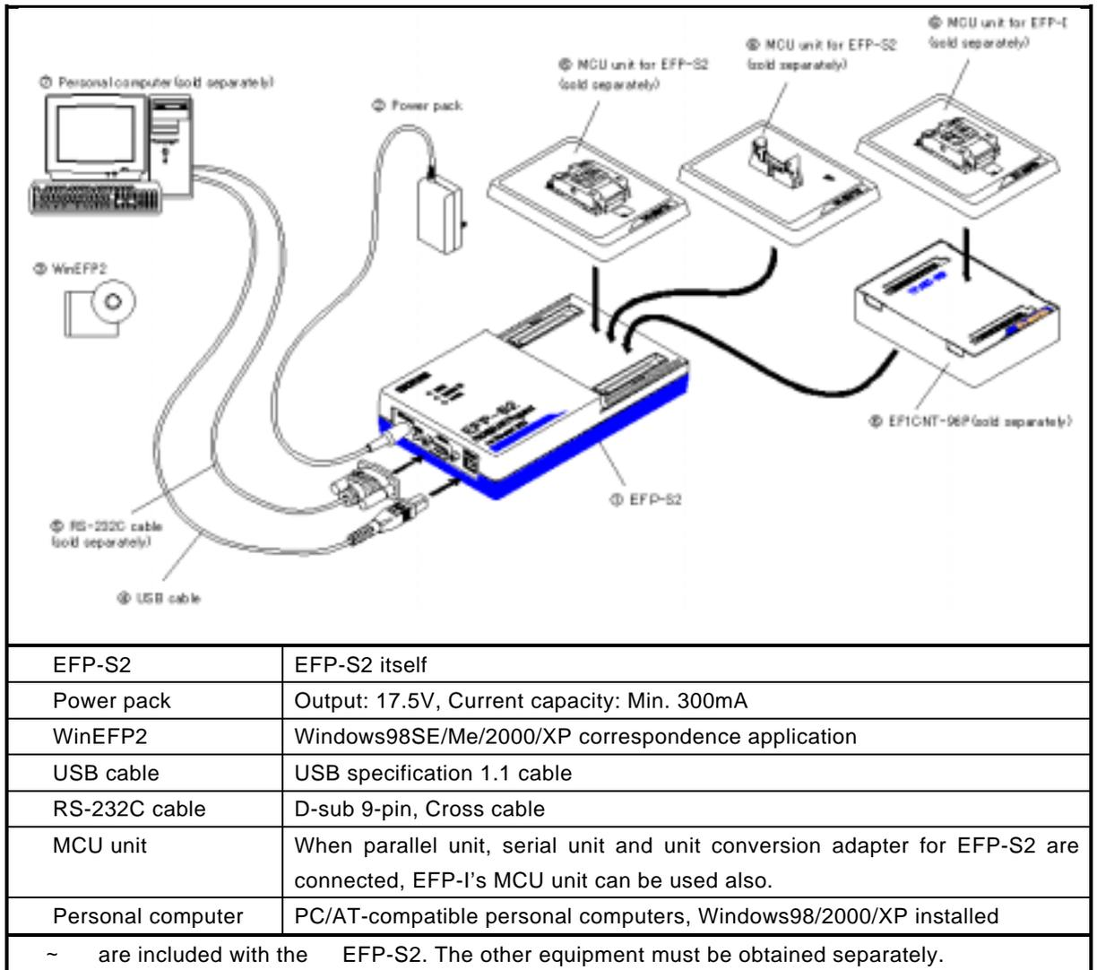
Fig. 2.1: System Configuration
