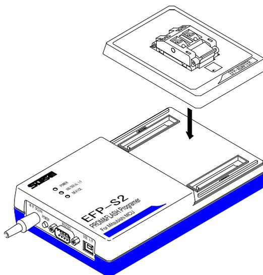
Fig. 1.1: MCU Unit Mounting Method
