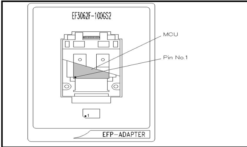
Figure 2.1: Pin Orientation of The socket
