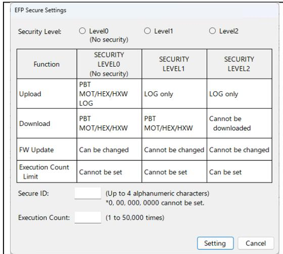
Figure 4.18 EFP Secure Settings
