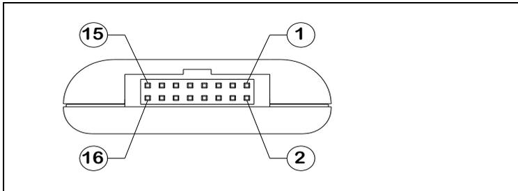
Figure 1.4 Connector pinout diagram for connecting to the target system
