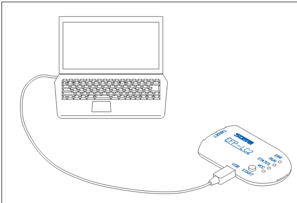
Figure 1.2 Connecting to the host machine
