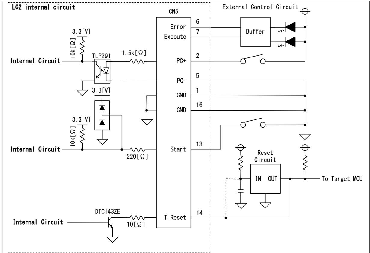
Figure 1.5 Example of external control signal connection
